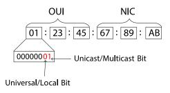
Figure 4.1: 48-bit MAC Address Structure
