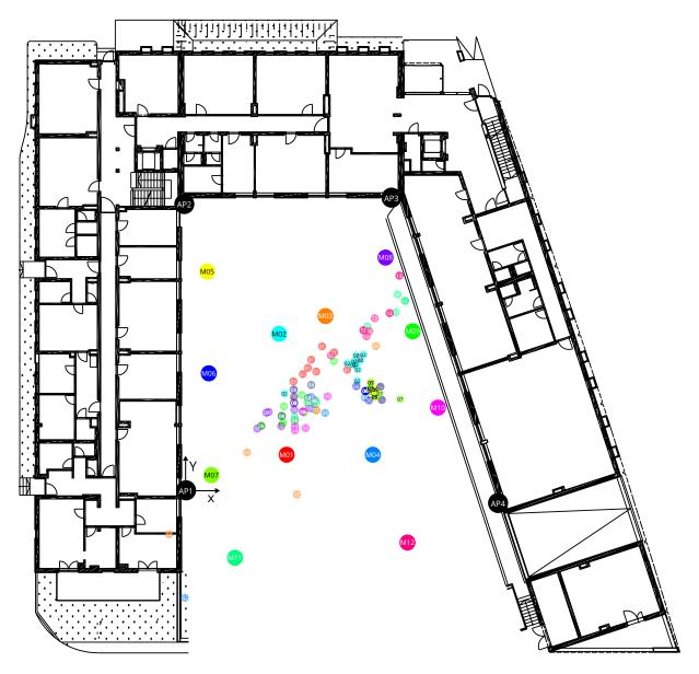
Figure 4.5: Position Estimation by RSSI Measurements – Result Visualization
